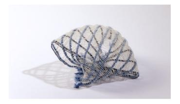
Textile designer Tiffany Loy teams up with SUTD's DManD (Singapore University of Technology and Design's Digital Manufacturing and Design Centre) to explore advanced automated textile construction as a means of additive manufacturing.
